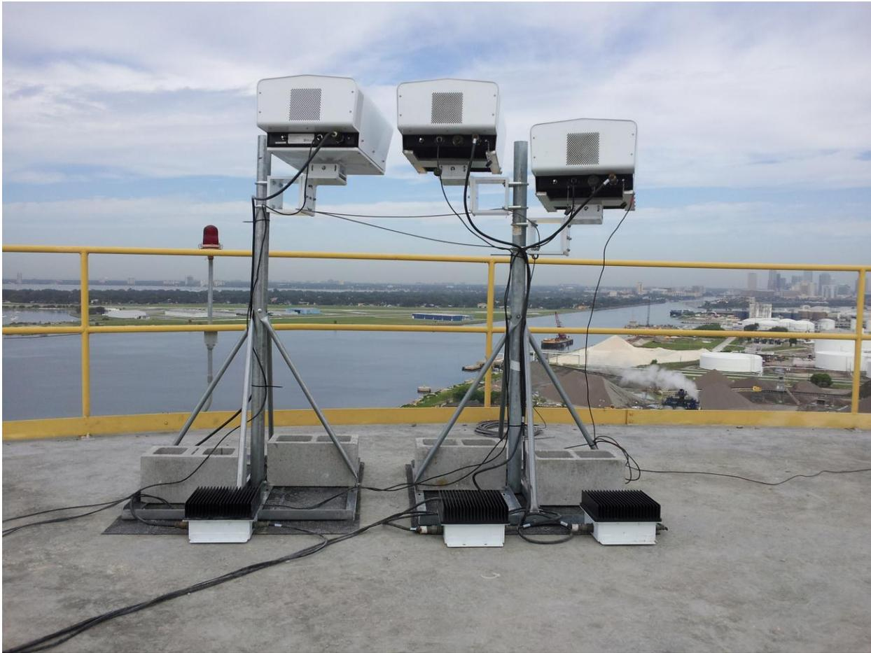
*Install of LWIR, MWIR and VIS cameras on a non-penetrating roof mount.*
