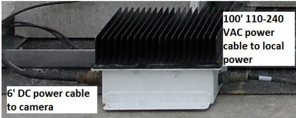
The cameras and servers require 110VAC – 240VAC, 50Hz – 60Hz. The input power must be properly grounded and conditioned to protect the equipment from low voltage, fast transients and other anomalies that might harm the equipment. Each camera comes with an external power supply which must be mounted within 6' of the camera.
